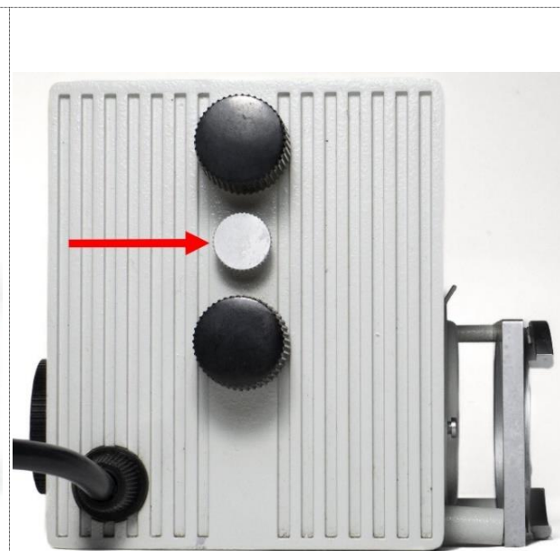
Figure 4: The left-side panel. The red arrow points to its locking screw knob.
