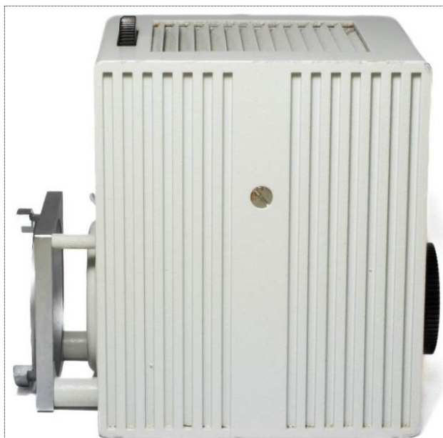
Figure 3: The right-side panel with its locking screw.
